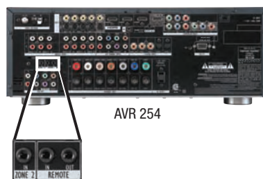
Figure 38 – IR Inputs and Outputs
