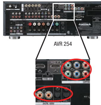
Figure 25 – Connecting a Component-Video-Equipped Recorder
