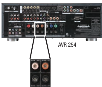
Figure 39 – Surround Back/Zone 2 Speaker Outputs
