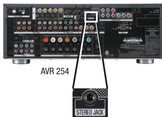
Figure 30 – Connecting a Portable Audio Player
