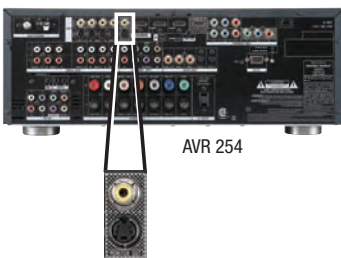
Figure 34 – Composite and S-Video Monitor Outputs
