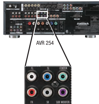
Figure 21 – Connecting a Multichannel Audio Player
