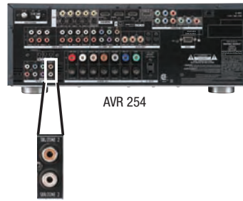
Figure 40 – Surround Back/Multizone Preamp Outputs
